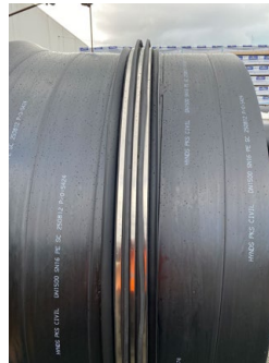
FIG. 2 Stub Flange connection type
